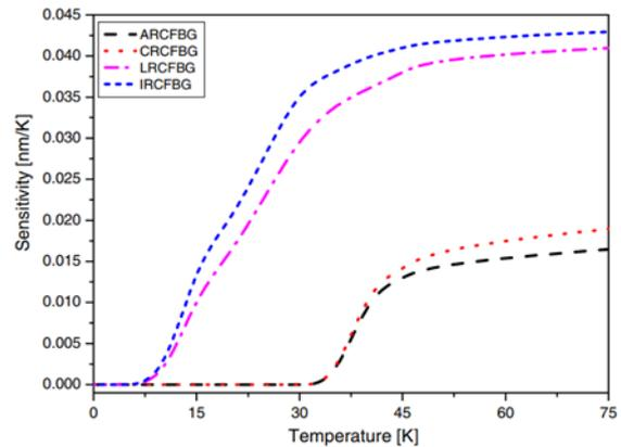
Fig. 1. Sensitivity of different metal-coated FBG sensors
