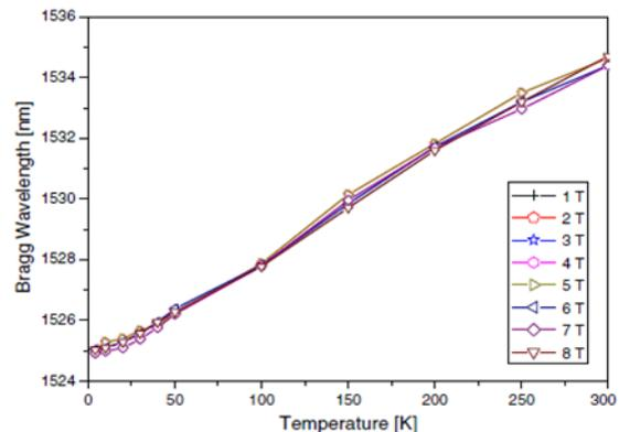
Fig. 2. IRCFBG sensor responses for varying magnetic fields
