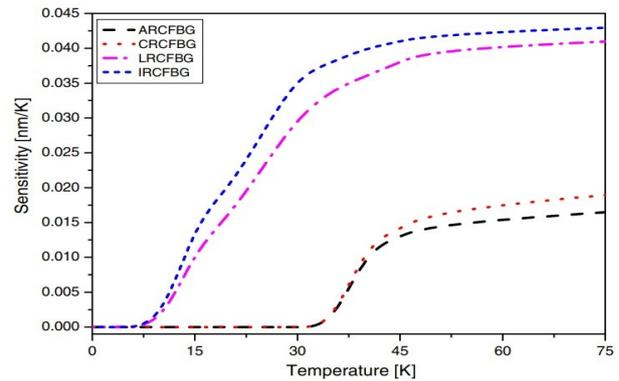
Fig. 1. Sensitivity of different metal-coated FBG sensors
