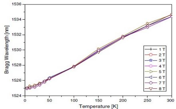
Fig. 2. IRCFBG sensor responses for varying magnetic fields
